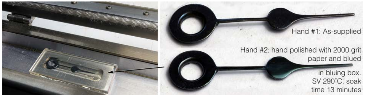
Figure 22 Comparison of a professionally blued hand (upper right) with one blued in the bluing box (lower right)
