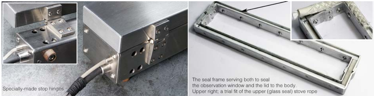
Figure 12 Further details of the bluing box
