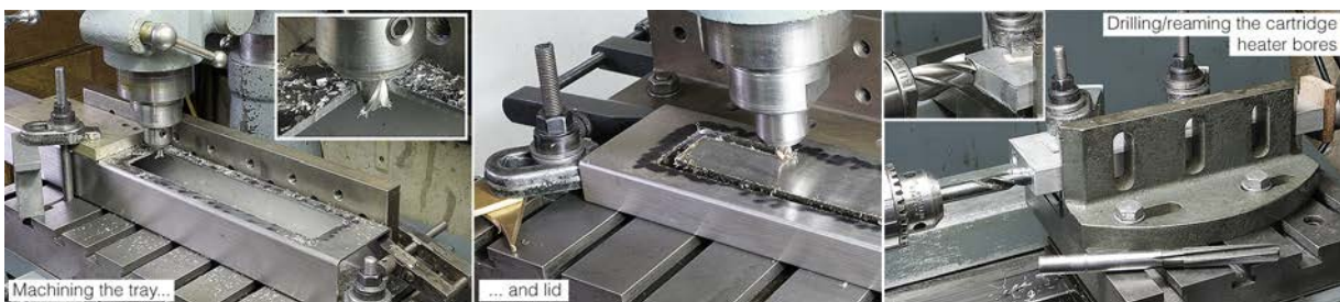
Figure 11 Cutting the openings in the stainless steel RHS, and (right) drilling the hotplate for the cartridge heaters
