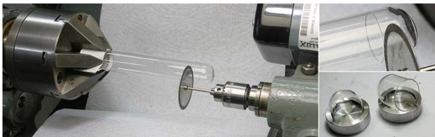
Figure 17 Cutting a borosilicate chamber from a test tube
