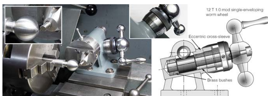
Figure 25 The author's spherical turning attachment
