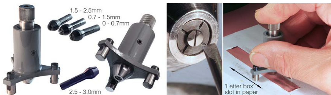
Figure 2 The author's screw head polishing tool
