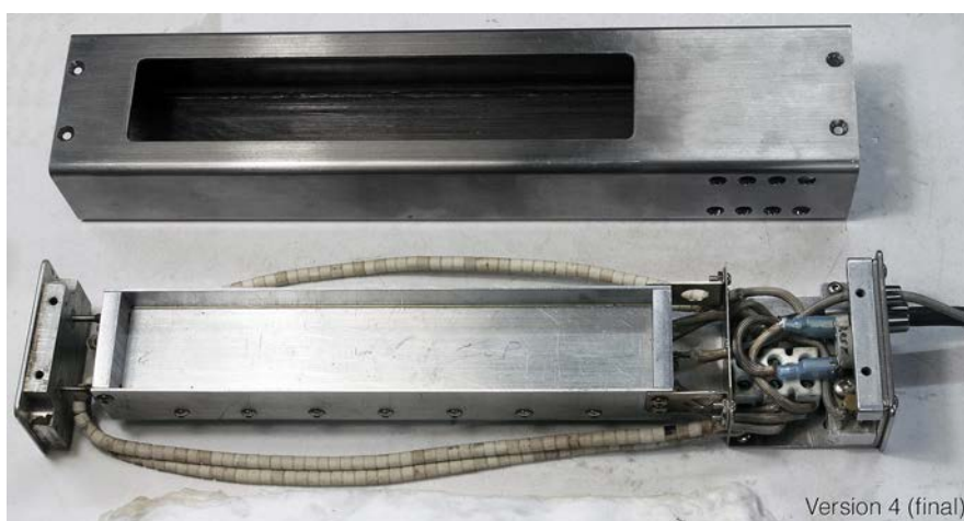
Figure 9 The lower part of Version 4 of the bluing box
