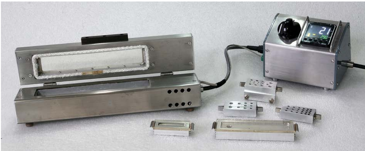
Figure 6 Version 4 of the author's PID-controlled bluing box and accessories
