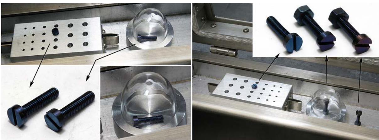
Figure 18 Comparison of the results of bluing screws using a block and chamber with the screws in differing orientations
